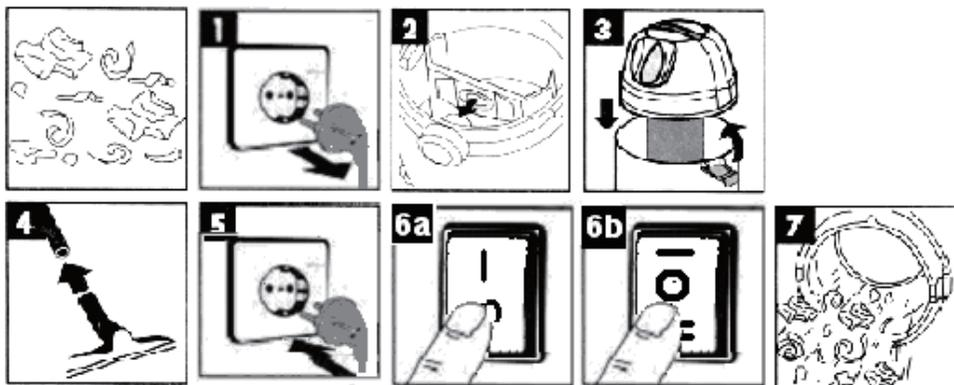
Unplug before change filter or dust partition bag (Figure 1), then take out the bag and empty the dust or replace the bag. Slip the dust bag onto the socket (figure 2) for dry vacuum-cleaning.
